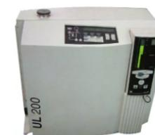
Helium Leakage Detector
